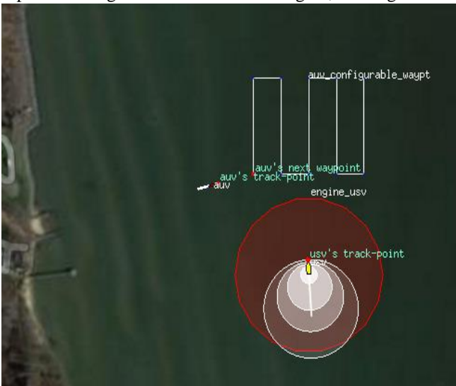
Figure 5: Surface vessel transiting through AUV search area. The red circle indicates the range of the vessel's engine noise, and the white circles represent active pings from the vessel.
