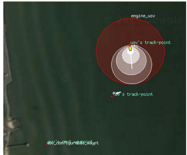
Figure 6: The AUV returning to a safe point after detecting the surface vessel's pings
